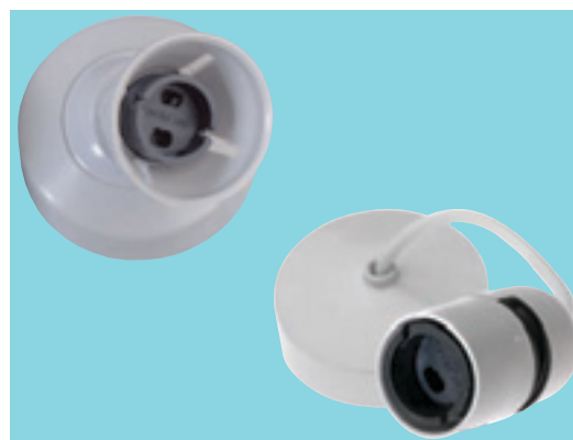
The safety Lampholder has a unique shutter action which ensures that when a lamp is removed the contact pins are retracted and shielded making them inaccessible to touch.
